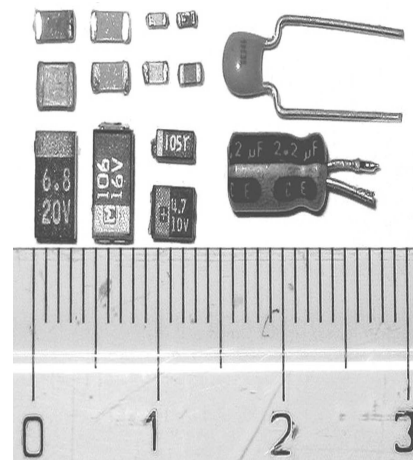
FIG. 1-12. Chip and ceramic capacitors. (Courtesy of Wikipedia)
