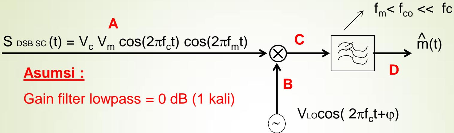
$$S_{\text{DSB-SC}}(t) = \left( \frac{V_c V_m}{2} \right) \cos 2\pi(f_c + f_m)t + \left( \frac{V_p V_m}{2} \right) \cos 2\pi(f_c - f_m)t$$
