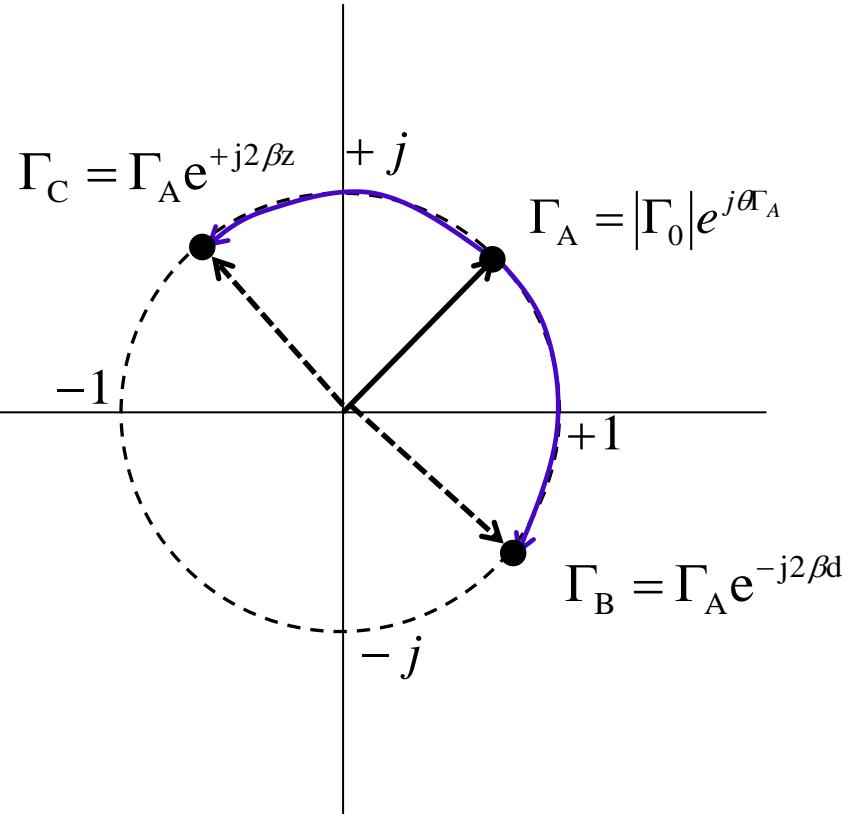
$$V(z) = V^+(z) + V^-(z) = V^+(z) + V^+(z)\Gamma_v(z)$$
