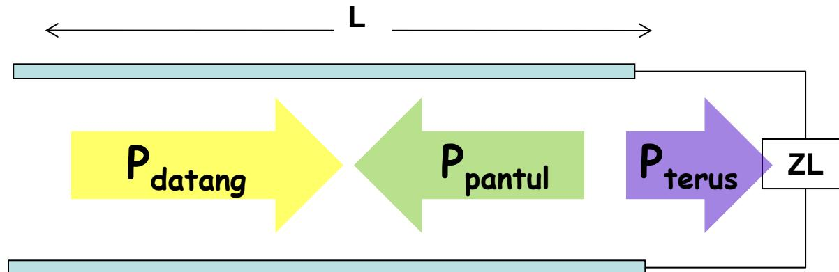
$$\begin{aligned} \text{Missmatch Loss}(z) &= \frac{P_{\text{terus}}}{P_{\text{datang}}} = \frac{P_{\text{datang}} - P_{\text{pantul}}}{P_{\text{datang}}} = \frac{P_{\text{datang}} - P_{\text{datang}}|\Gamma_v(z)|^2}{P_{\text{datang}}} = \frac{P_{\text{datang}}(1 - |\Gamma_v(z)|^2)}{P_{\text{datang}}} \\ &= 1 - |\Gamma_v(z)|^2 \end{aligned}$$
