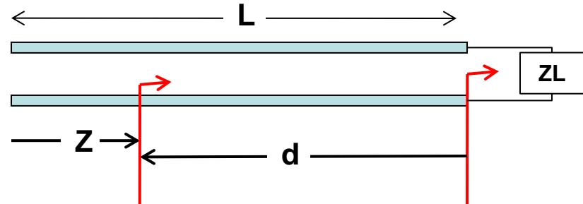
$$\begin{aligned} \Gamma_v(d) &= \left( \frac{Z_L - Z_0}{Z_L + Z_0} \right) e^{-2\alpha d} e^{-j2\beta d} \\ &= \left( \frac{Z_L - Z_0}{Z_L + Z_0} \right) e^{-j2\beta d} \Rightarrow \text{Lossless} \end{aligned}$$
